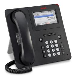
The 9621G IP Deskphone has a graphical color display, large touch screen and integrated Gigabit interface. Part of the 9600 Series IP Deskphones, the 9621G leverages your enterprise IP Network to deliver sophisticated voice communications from headquarters. remote locations or home offices. Integrated with the Avaya Aura® and IP Office™ Platforms, the 9621G optimizes communications through a flexible architecture that leverages existing investments and accommodates changing business needs.
