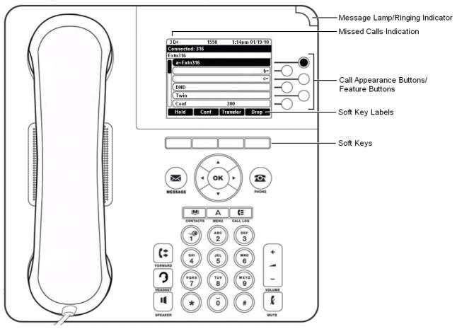
The phone supports 24 programmable call appearance/feature buttons. The labels for 6 of these are displayed in the main display and can be controlled by the adjacent buttons to the right. You can use the ▲ up/down ▼ keys to scroll the display. You can also use the ◀ left/right ▶ keys to move through the button feature in pages of 6.
